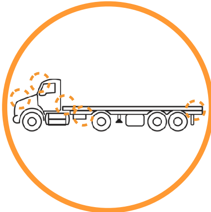
7 EXTERNAL LIGHTS AREA
